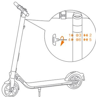
2. Firmly connect the wires inside the handlebar and the stem. Slide the handlebar onto the stem. Be aware of the correct orientation.
