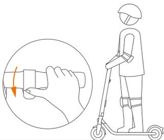
3. Put your other foot on the foot deck to keep both feet stable. Press the throttle to speed up when you are balanced.
