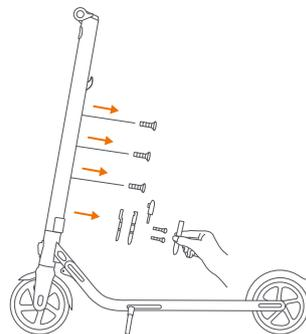
3. Install the external battery on the rail and fix it with the M4 (20mm) screws (2 pcs) and M3 screw (1 pcs), provided with this product. After they are properly installed, block the screw holes with the rubber stopper.
