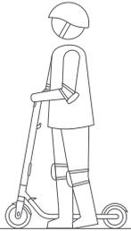
**!** DO NOT press the throttle when walking with the scooter.
