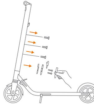
3. Install the battery pack onto the support bracket and tighten the screws securely.
